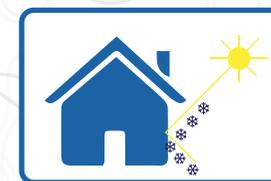
The application of Thermogel Paint allows the solar radiation falling on the building to be reflected, keeping the interior temperature cooler and promoting energy savings. In winter, the warmth generated by the heating system also remains inside the building for longer.
